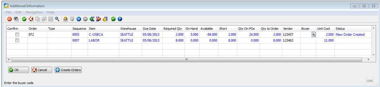
The PO number created will then display on the Component Screen. The available and on hand are null to show that the component quantity will be supplied by the purchase order.
